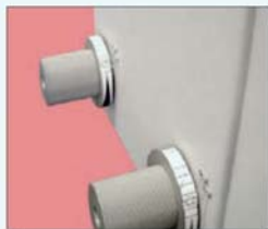
Nip & Pull Roller Adjustment
