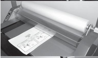
Slide the top and bottom film rolls from side to side on the mandrels so that the film is perfectly aligned top and bottom (Note: overlap will cause the film to deposit residue on the heat shoes and rollers, so this procedure is critical). Replace feed tray and heat guard.
