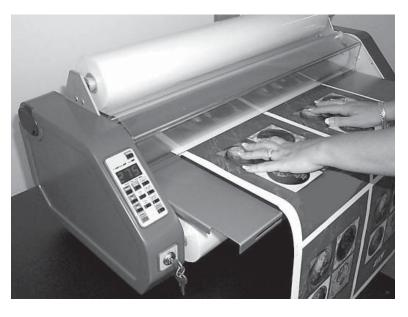
rear rollers, allow 3" to 6" of film to clear the rollers at the end of your document and turn the motor switch to stop. Using the hand held cutter, hold tension on the laminated document and slice through the film to release the document. Multiple documents can be run successfully if desired and cut at a later time.
