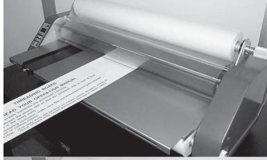
Start the motor by pressing the "Start" button, and reduce the speed to 1 foot/min. Feed the threading board and film in between the heat shoes. This will pull the film through the rollers until it comes out the back of the laminator.
