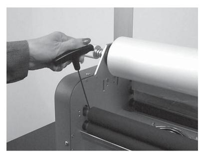
**Shut the machine off!** D&K Minikotes have set screws at both ends of each laminating and pull roller. With the use of a 3/32 hex key, loosen all four set screws on the pull rollers. Cut the plastic between the laminating and pull rollers, grab the loose end and pull. The rollers will rotate freely on the roll shafts and the "wrap-around" will easily unwrap. Tighten all the set screws and rethread the film.
