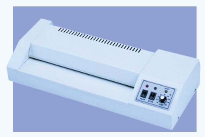
The Tamerica Tashin TCC 330 Pouch Laminator with a 13" wide laminating throat is an ideal pouch laminator for medium use office laminating environments. This pouch laminator is capable of laminating letter, legal and menu size documents in laminating pouches up to 10mil in thickness. This pouch laminator features a quick warm up time of 3.5 to 4.5 minutes along with a lamination speed of 14" per minute.
