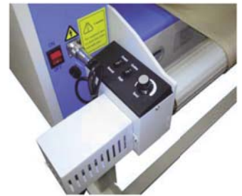
Motorized rear rewind for roll-to-roll applications
