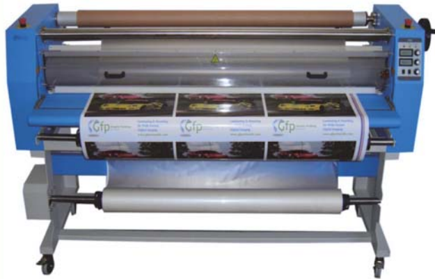
Two front unwind shafts for roll-to-roll encapsulation.
